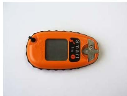
Figure 12. Digital fence volt meter.
