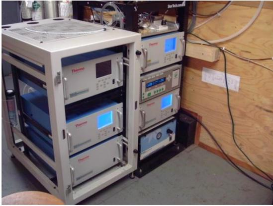
Gas analyzers for NH<sub>3</sub>, H<sub>2</sub>S, CH<sub>4</sub>, N<sub>2</sub>O, & CO<sub>2</sub>
