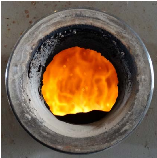
Figure 3. Flame from the combustion of the gasifier-generated syngas inside the combustion chamber.
