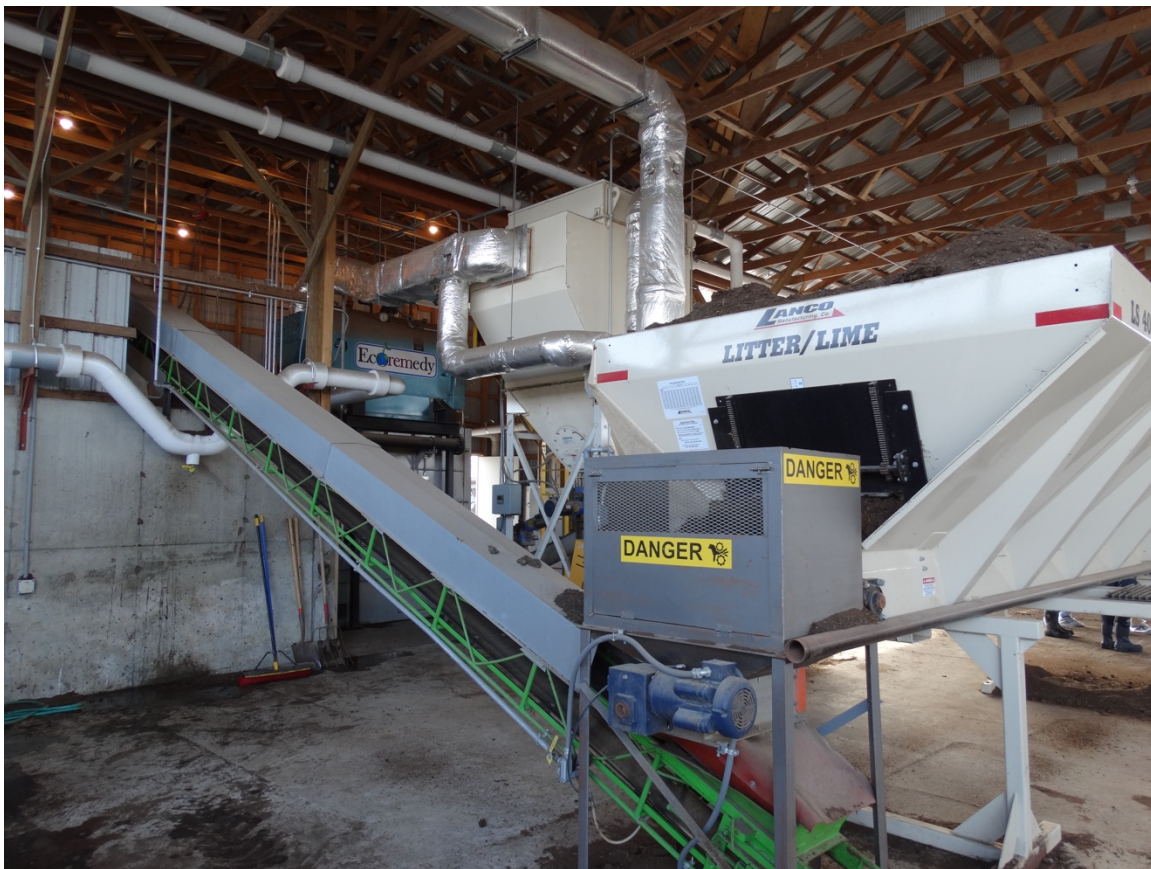
Figure 1. Litter starts in the litter spreader (white piece of machinery) that goes through a lump breaker (grey piece labeled “Danger”) and then is conveyed to a hopper above the gasifier (hopper not pictured).
