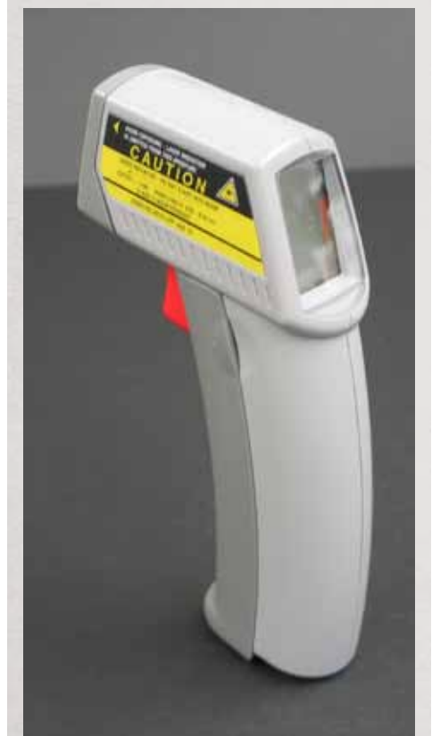
Figure 8. Examples of infrared camera (top) and thermometer (bottom) for surface temperature evaluation
