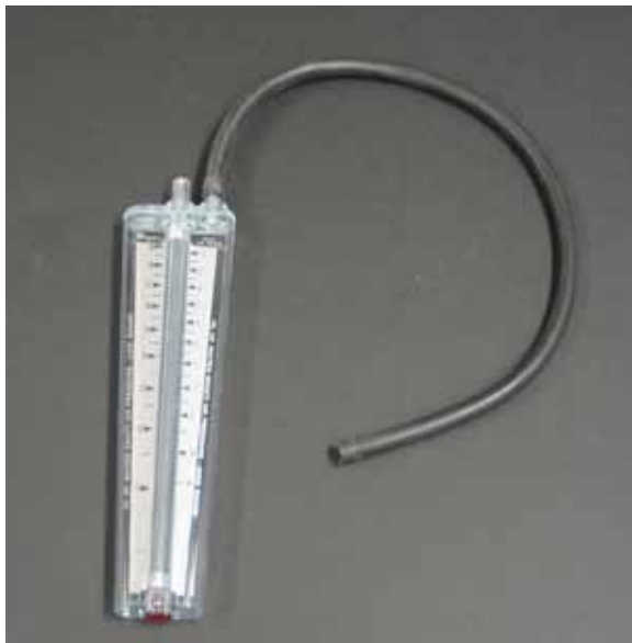
Figure 12. An example of a static pressure bubble meter (manometer)
