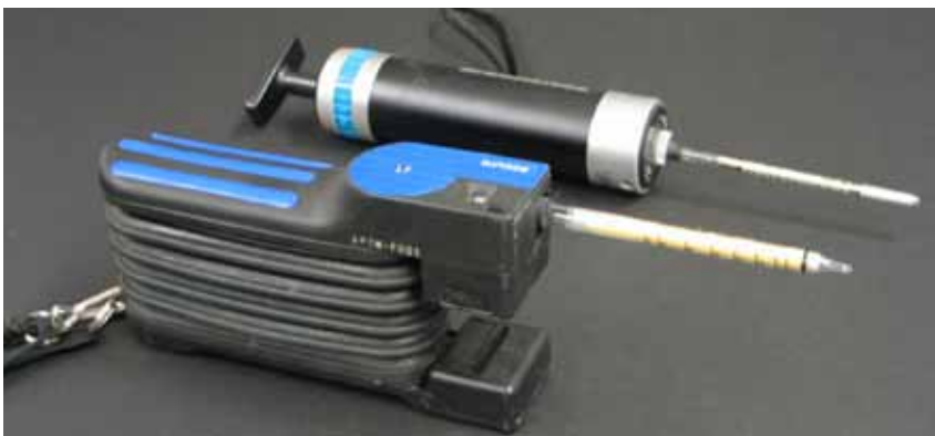
Figure 9. Examples of handheld sampler pumps and colorimetric tubes to measure gas levels
