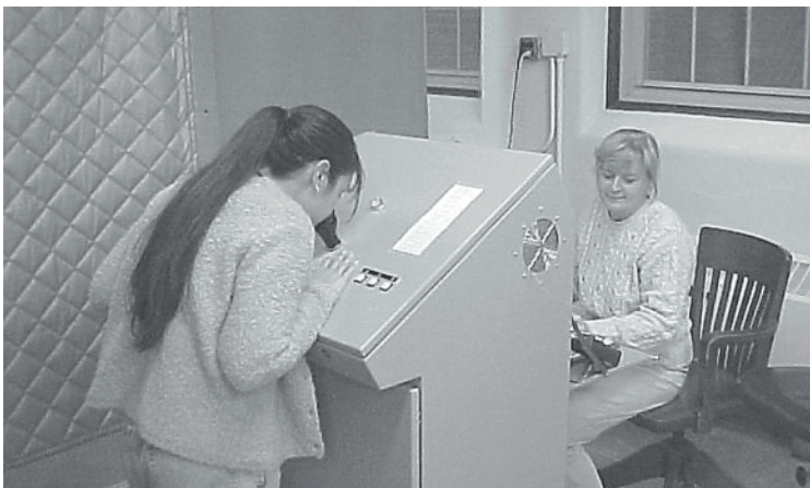
Figure 40-11. Panelist, olfactometer, and panel leader.
