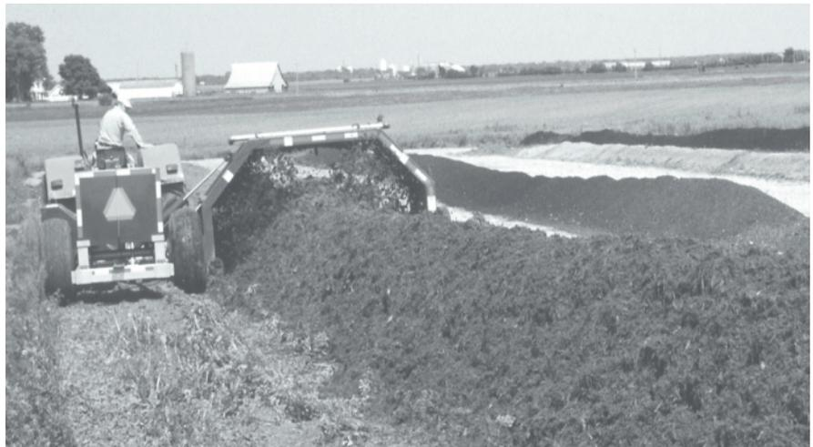
Figure 44-7. Mechanical turner used in composting solid manure.
