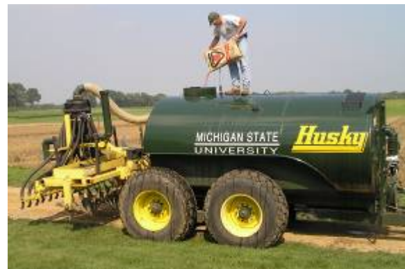
Figure 2. The seed was added to the manure slurry in the tank. Bypass flow provided tank agitation for seed mixing and distribution.
