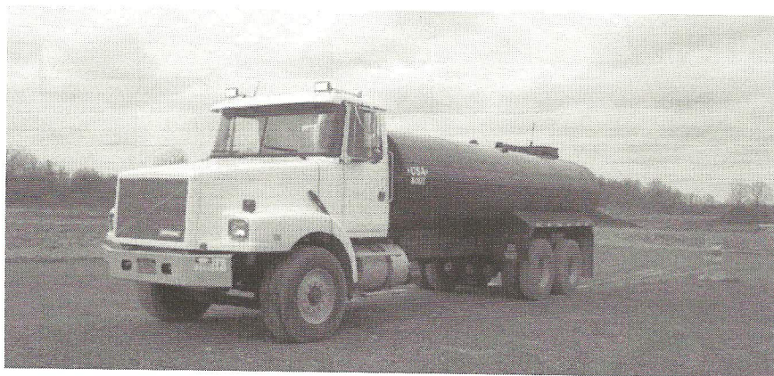
Figure 2. 4,500 Gallon tanker truck used for hauling manure to site and digested effluent from site
