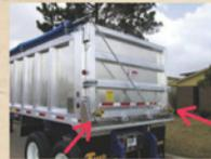
Ball valve drains, in gate or underbody
