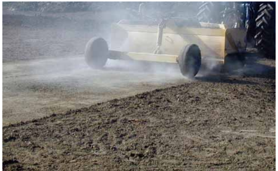
Figure 3. Box blades are effective at maintaining a smooth, hard pen surface without gouging the interfacial layer and exposing mineral soil. The manure being harvested in this photo will have a higher heating value of about 5,000 Btu/lb as collected and would be considered a relatively high-value biofuel feedstock. (Photo: S. Sakirkin)
