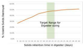
Biogas production is a function of manure quality/quantity and retention time
