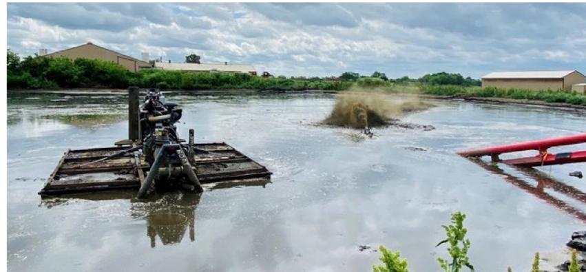
PTO-drive lagoon agitators and agitation boat in operation.
