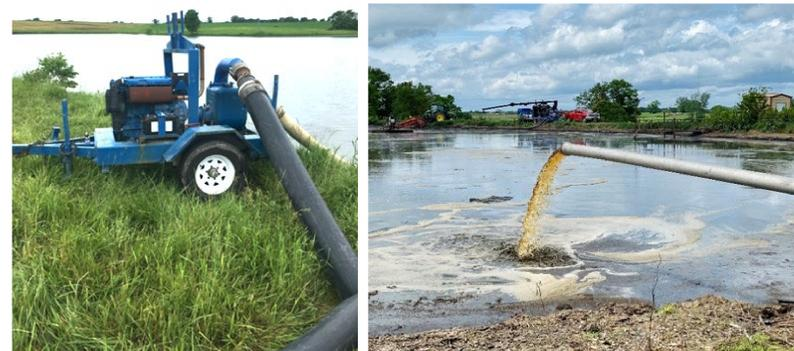
A dilution pump was used to pump water from the nearby lake (left) to the dairy lagoon (right) with agitation boat and lagoon agitation working in the background.
